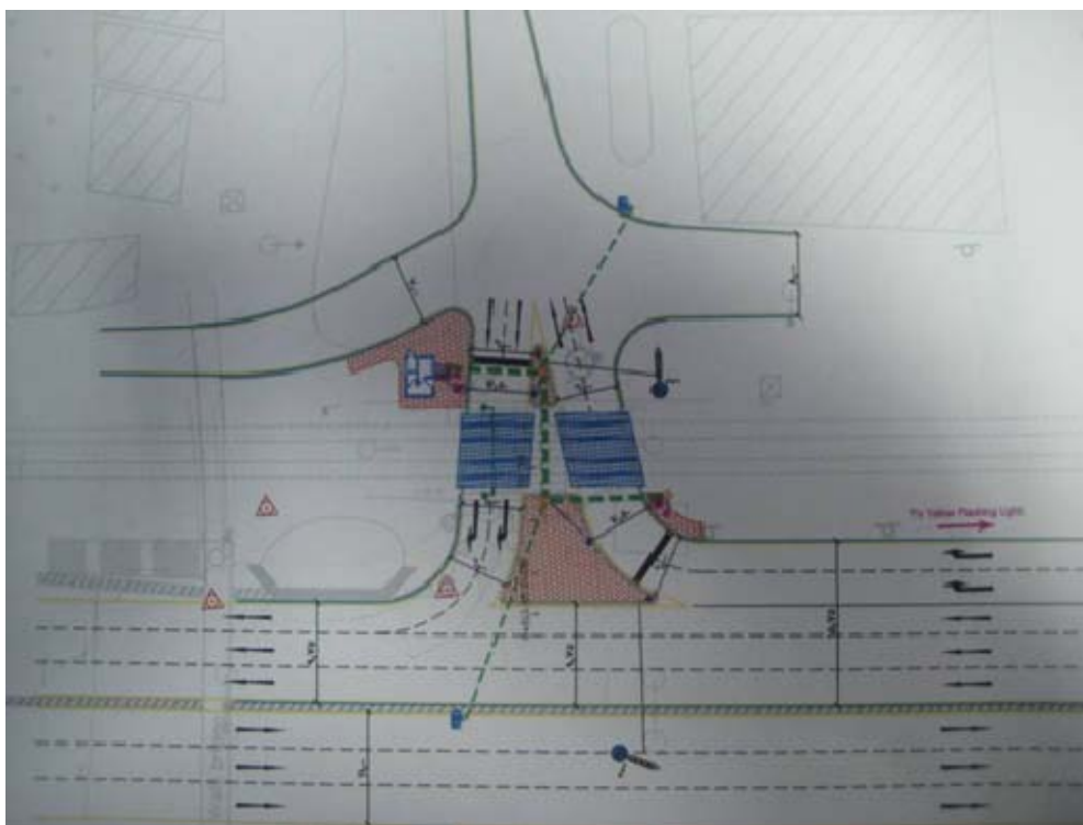
Example of a design plan with missing acceleration lane and unclear organisation of the merging traffic
